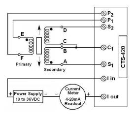
A through F: Connector pin assignments
